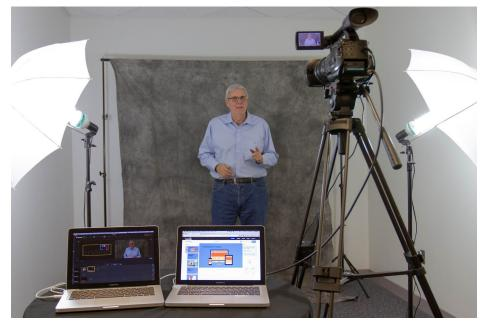
This is a typical small studio setup for Knovio Live. The left-hand laptop is running Telestream's Wirecast, a software-only switcher/encoder, which turns the camera's video signal into a stream that can be digested and broadcast globally through Amazon's MediaLive platform. The right-hand laptop is running Knovio, and controls the synchronization of all the slides and other on-screen materials. Wirecast and Knovio can be run, if desired, on the same computer.
