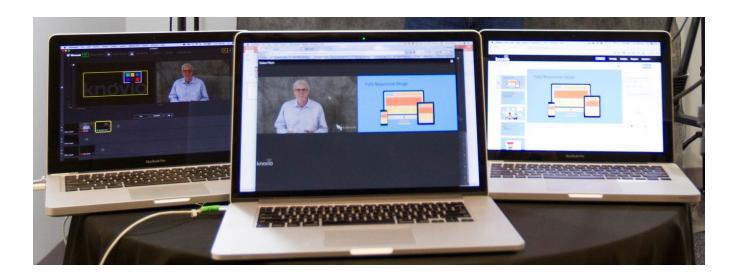
The Knovio Smart Player (center, above) takes the video stream from Wirecast and Brightcove and presents it side-by-side with synchronized slides and images from Knovio. A patent-pending process maintains the synchronization, even if network congestion or other factors cause delays or buffering in the video stream. This live multimedia webcast can be viewed on any desktop, laptop, or mobile browser.
