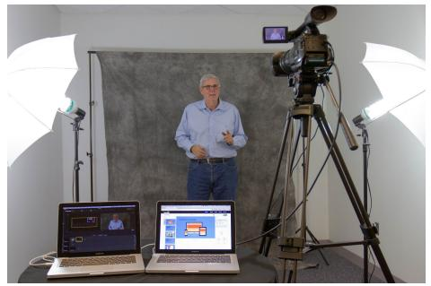
This is a typical small studio setup for Knovio Live. The left-hand laptop is running Telestream's Wirecast, a software-only switcher/encoder, which turns the camera's video signal into a stream that can be digested by Brightcove's Live Module and broadcast globally. The right-hand laptop is running Knovio, and controls the synchronization of all the slides and other on-screen materials. Wirecast and Knovio can be run, if desired, on the same computer.
